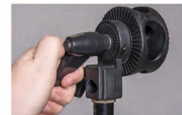
Begin by mounting the cam onto the COR752 light stand and securing it into place. Then, loosen the cam grip by turning the Tilt Adjustment Knob counter-clockwise (you may need to gently pull apart the two halves of the cam to open).
