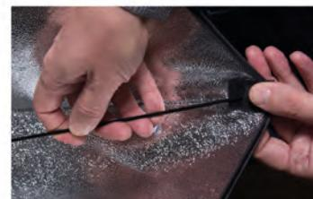
Beginning with the top left corner, place one end of the softbox rod into the lamp head. Pull the top left corner of the softbox over the rod and insert the silver rod tip into the black pocket in the corner of the softbox. Continue by repeating this process for the remaining three rods.
